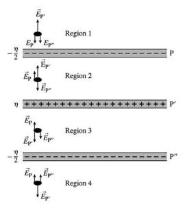
From planar symmetry the electric field can point straight toward or away from the plane. The three planes are labeled as P (top), P', and P"(bottom).
