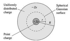
The nucleus is a positive point charge +Ze at the center of a sphere of radius R. The spherical symmetry of the charge distribution tells us that the electric field must be radial. We choose a spherical Gaussian surface to match the spherical symmetry of the charge distribution and the field. The Gaussian surface is at r < R, which means that we will calculate the amount of charge contained in this surface.
